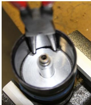
Once the plate is seated, reinstall the snap ring and make certain it is fully seated in the groove.
