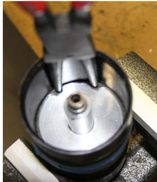
Once again, it's often easier to remove the 2 lower piston plates and shaft by using air pressure to dislodge the assembly. Connect the tool to the air source and let the air pressure push the assembly up,
