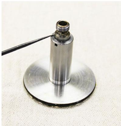
The power pack end cap also has 2 O-rings. Replace and lubricate with light machine oil or grease.
