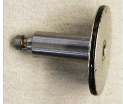
The lower piston shaft also has a small O-ring located “inside” the shaft. Replacing this internal O-ring can be a challenge, but it should always be replaced as it is often the O-ring that is causing air leakage. The pointer in the image below shows the location of the O-ring inside the shaft.
