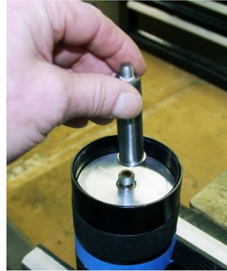
Once the upper shaft has been removed, you can now remove the upper piston plate. It's often easier to connect your air source (40-60 psi) and let the air pressure dislodge the piston plate. Reconnect the tool to your air source and the upper plate should dislodge as shown below.
