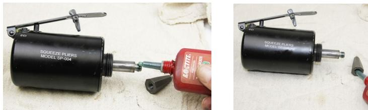
Once the thread sealant has cured, reposition the tool in the vise to vertical and check the end cap for tightness. This cap does NOT need to be torqued down too tight. Over-tightening the end cap may make it more difficult to remove in the future.
